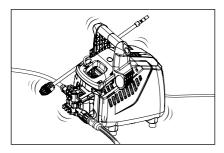
Having closed the trigger gun with safety catch, the HP cleaner must shut down. Failure to shut down may be caused by leakage in the pump, the pressure switch, the high pressure hose or the trigger gun with safety catch.
