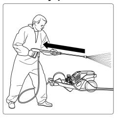
Bear in mind that during cleaning tasks with a high-pressure water jet a significant recoil at the lance arises (see technical data on page 4).
