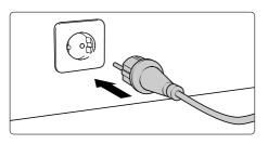
**11.** Connect to circuit. The socket must be protected with a 16A delay action fuse on the mains side.
