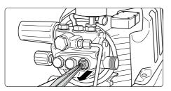
Take out valve body (with green or red plastic coating) and O-ring by means of needle nose pliers. Check O-ring for damage. In case of a damage the O-ring has to be replaced.
