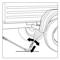
Always aim the underbody lance! Bear in mind when using a curved or angled spraying lance that there is a significant amount of torque in the recoil!
