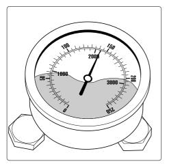
The pressure gauge shows full pressure, but from the nozzle comes only little water or no water at all.
