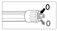
Unscrew HP hose, gun and lance and check the O-rings.
