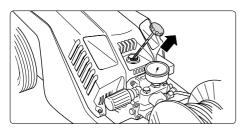
3. Each time check oil level at the oil dipstick prior to putting the HP cleaner into operation. (Take care that cleaner is in horizontal position!)
