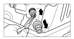
2. Check water inlet filter for cleanliness prior to putting the machine into operation!
