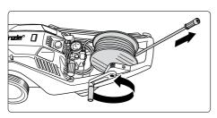
**9.** Put HP cleaner into horizontal position. These machines must be operated in horizontal position! Unwind HP hose from hose drum without kinks and nooses.
