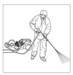
**13.** Ventilation of the machine: Pull and release the trigger several times. Switch on high-pressure cleaner with opened spray gun. Start cleaning task.
