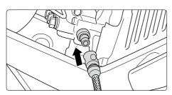
**10.** Connect water hose to water tank. The cleaner may be connected to water mains with cold or 60°C warm water. Alternatively water can be sucked in from a container (see page 17).
