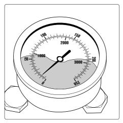
The pressure gauge shows little pressure despite fully turned up pressure regulation. The water from the lance comes in squirts. The HP hose vibrates.
