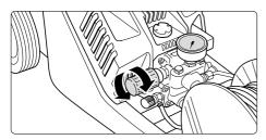
**12.** Steplessly adjust operating pressure with handwheel. The maximum pressure is adjusted ex work.
