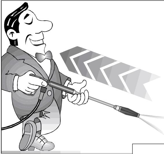
The recoil is less than 20 Nm.
