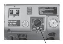
Thermostat with rotary control switch
