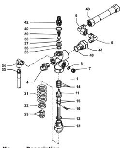
Safety valve for heating coil (Adjustment must be approx. 15% above the operating pressure)
